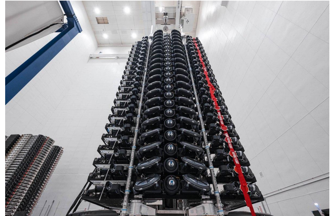
Stacked launch configuration of second-generation Starlink satellites (v2-Mini). (Credit: SpaceX)
