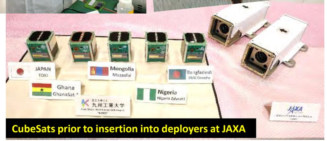
CubeSats prior to insertion into deployers at JAXA
