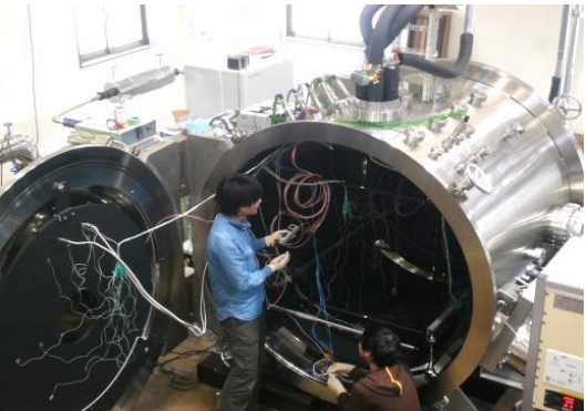
Thermal vacuum chamber at CeNT
