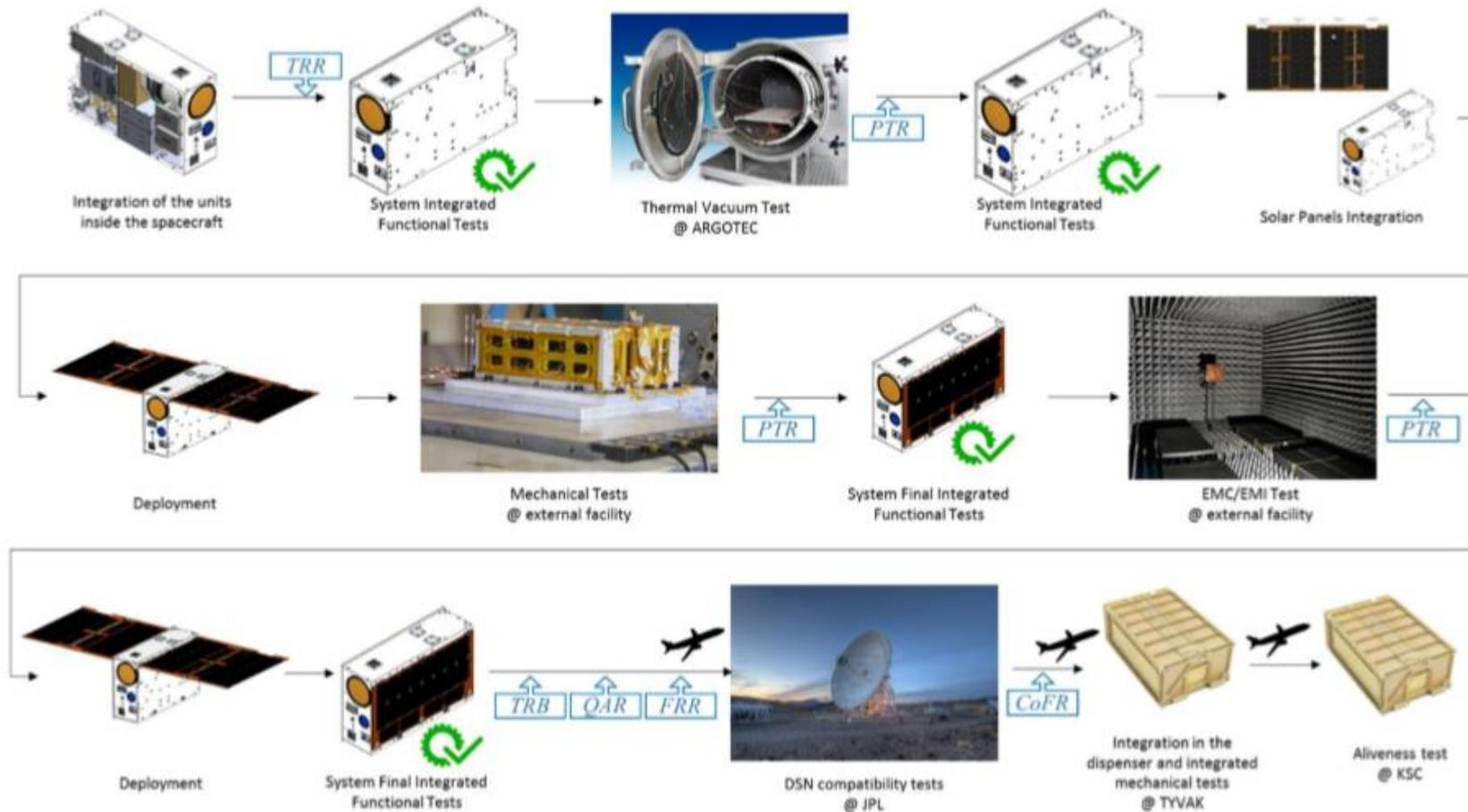
Proto-flight approach is implemented, before the delivery to Tyvak and integration in the dispenser.
