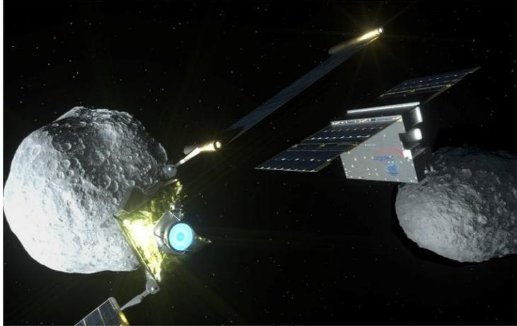
The **Light Italian Cubesat for imaging of Asteroids - LICIACube** will fly as piggyback of the **NASA-APL DART** probe towards the Didymos binary asteroid system, and will then be released to witness the impact effects of the American probe on the secondary Didymoon, in order to test trajectory deflection method by kinetic impact for Planetary Defense.
