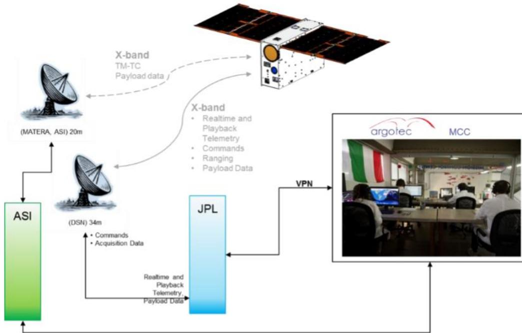
Communications based on X-band up and downlinks, with support of NASA DSN antennas and Italian facilities involvement, like the Sardinia Deep Space Antenna
