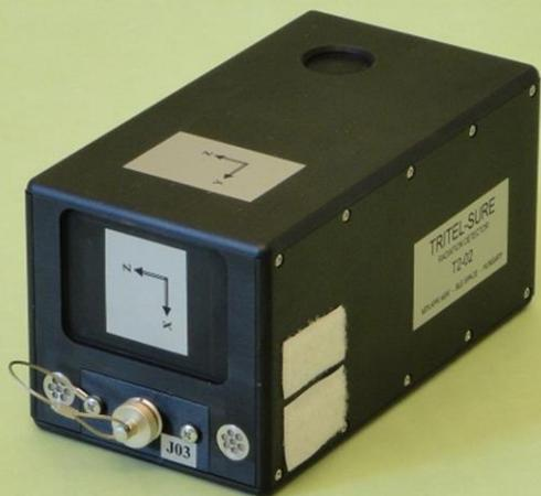
**TRITEL 3-dimensional silicon detector telescope system**
