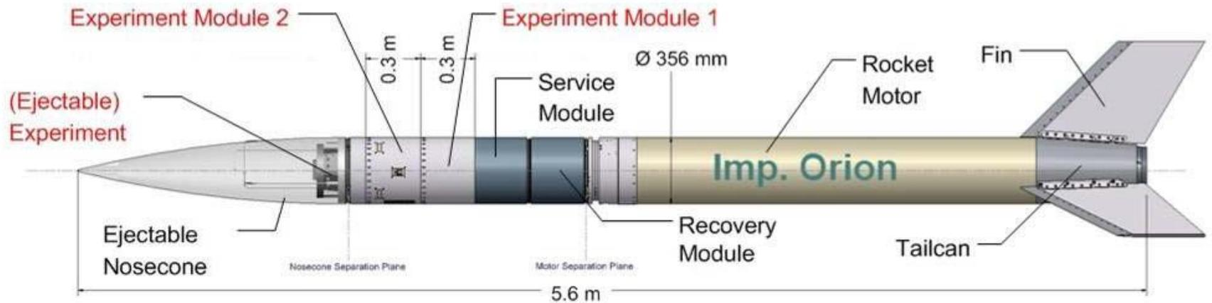
*Improved Orion rocket (REXUS system configuration)*
