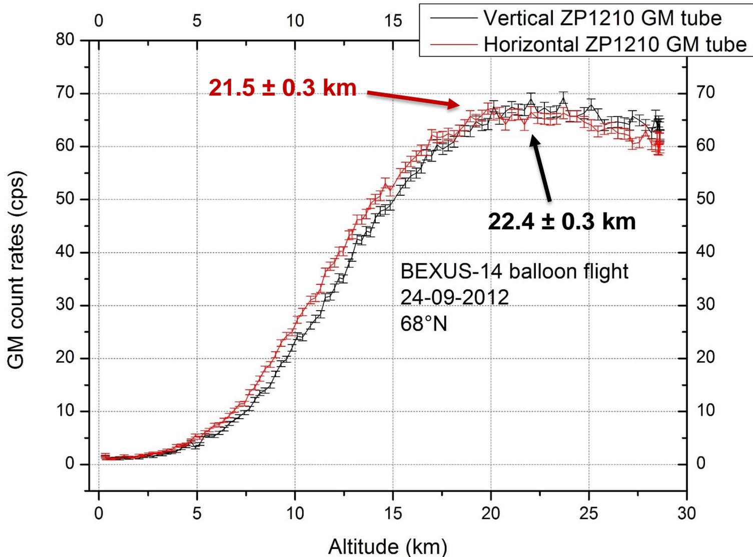
*Measured radiation profiles using ZP1210 type GM-tubes.*
