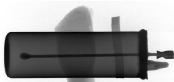
*GM tube internal structure in general*
