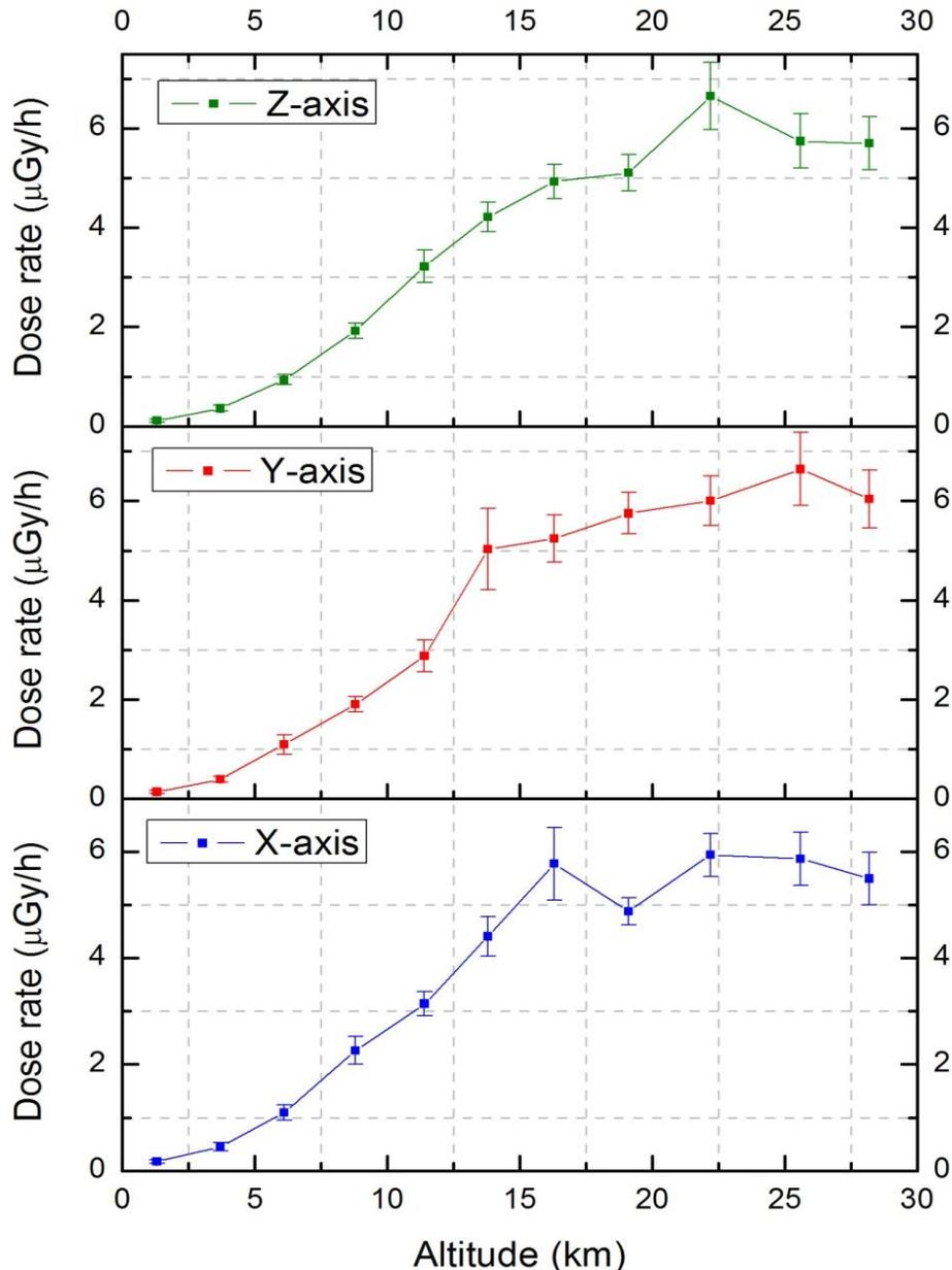
*Measured absorbed dose rates in water by TRITEL as a function of the altitude.*
