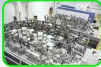
Structures hold mirrors and science instruments super stable, behavior must be known to ~38 nanometers (~1/10,000<sup>th</sup> of a human hair!)
