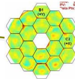
18 mirror segments computer controlled to operate as one mirror in space
