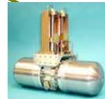
A cooler to chill the mid-infrared detectors to just 6 degrees above absolute zero.
