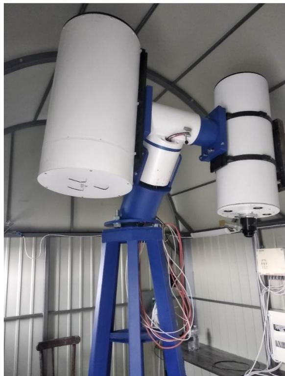
**Twin tube (0.35 m f/2.0 and 0.25 m f/12) telescope with CMOS cameras has been installed in Transcarpathian region. It will be fully operational by the summer of 2022.**
