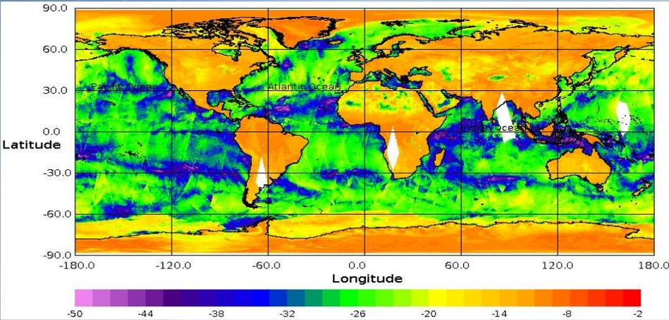
Outer-beam (VV) Backscattering coefficient (dB) from EOS-06 Scatterometer
