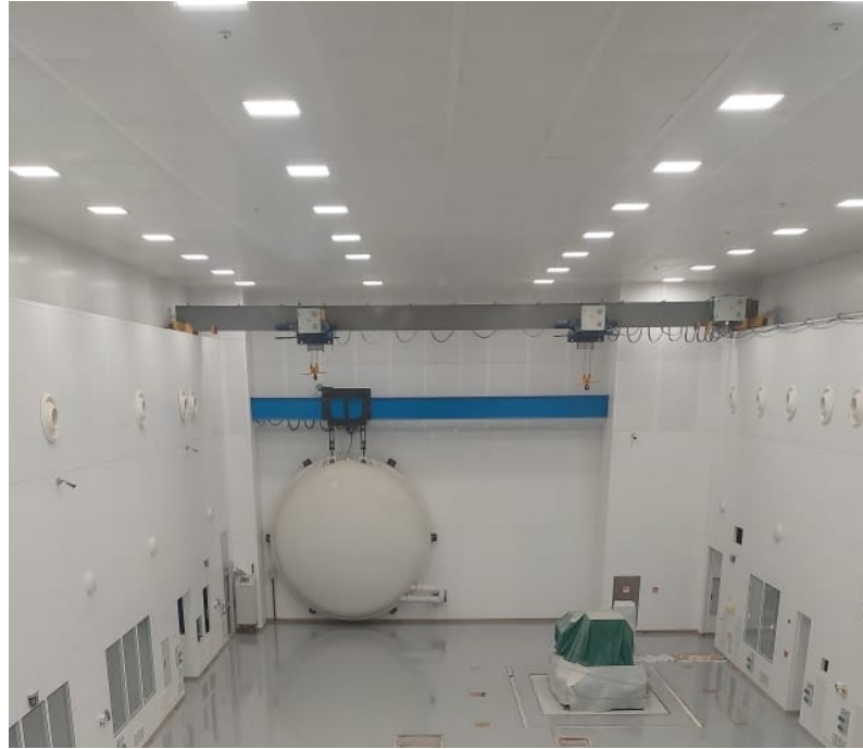
Thermal Vacuum Chamber for Satellite Environmental Testing Up to 600 Kg (Volume of Seattleite 1m 3 )
