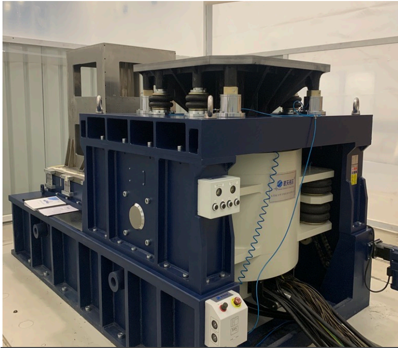
Shaker: Random, Sin and Shock Vibration Tests
