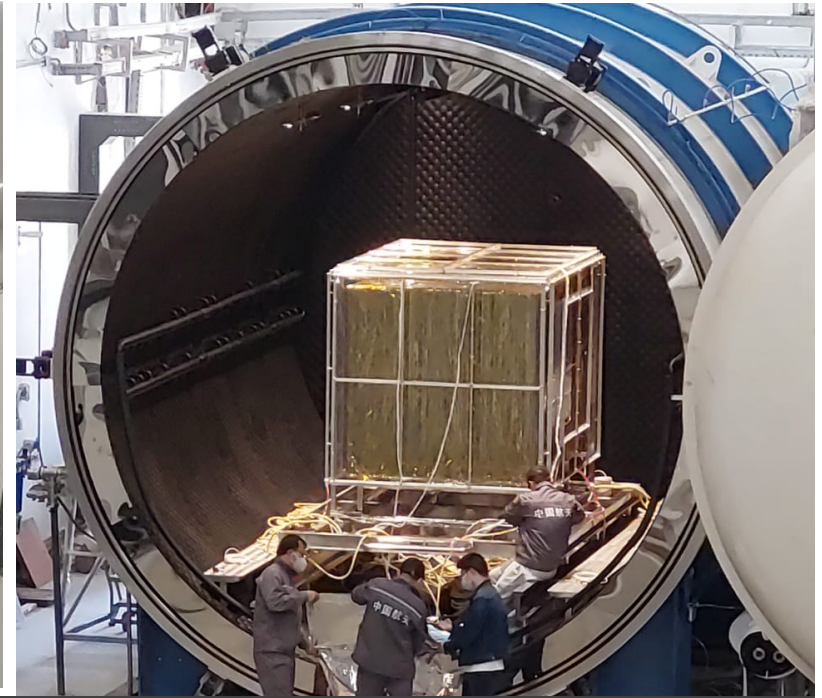
Thermal Vacuum Chamber for Satellite Environmental Testing Up to 600 Kg (Volume of Seattleite 1m 3 )
