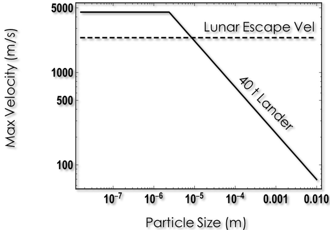
Model of maximum ejecta velocities as a function of lunar soil particle size.
