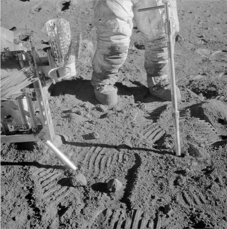
Lunar regolith is the **layer of unconsolidated rocks, pebbles, and dust** that exists on the lunar bedrock. The particles are sharp and angular in nature, resulting in a much more abrasive material than their terrestrial counterparts
