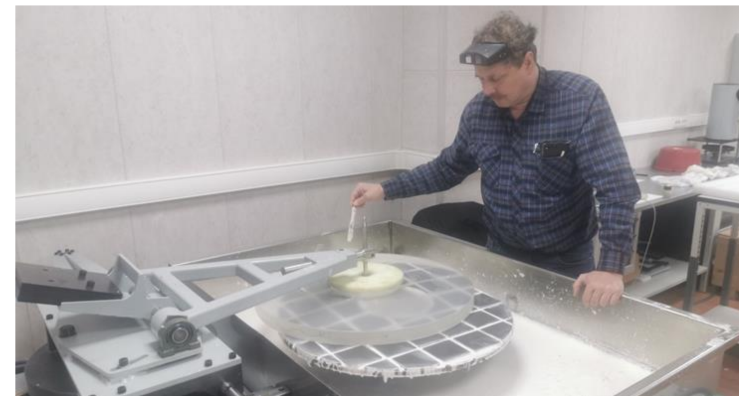
The grinding process of the full-aperture field corrector for WFOS-70
