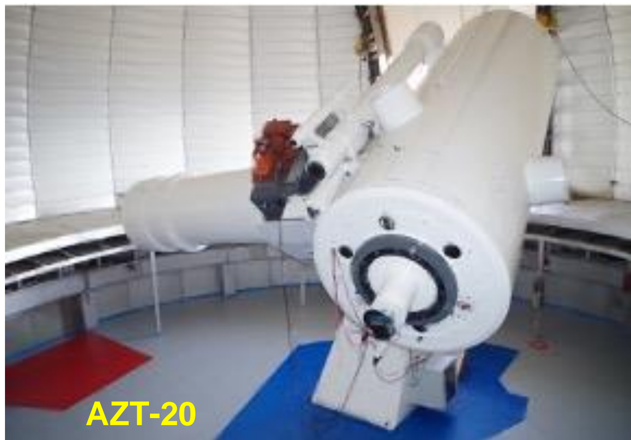
AZT-20 D=1560 mm, f = 1/3.8 , modified to operate in prime focus with 4-lenses quartz reducer D=280 mm, transparent in \lambda = 300 - 2500 nm, FOV = 60 \times 60 arcmin, 0.38''/\text{pix} , BVR "Astrodon". Remote control.
