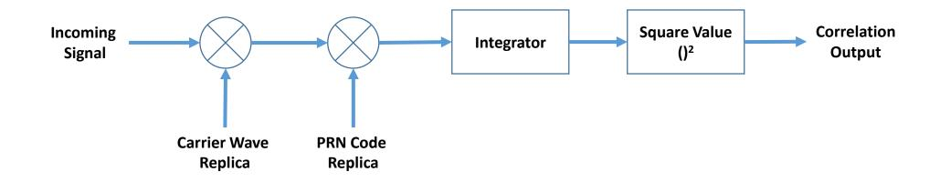
Identify visible satellites with coarse Doppler and Code Phase
