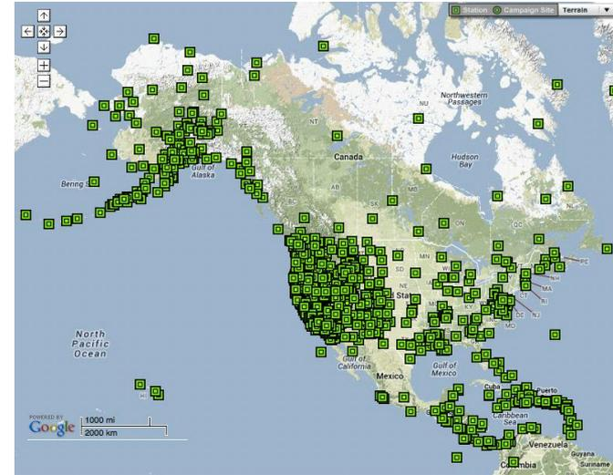
*PBO and Cascadia: 1632 Continuous GNSS Stations in operation (Fall 2014)*
