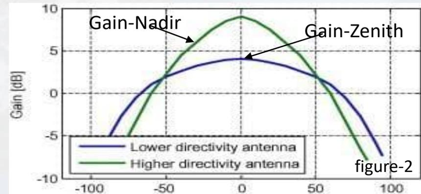
GNSS Transmitting antenna gain pattern
