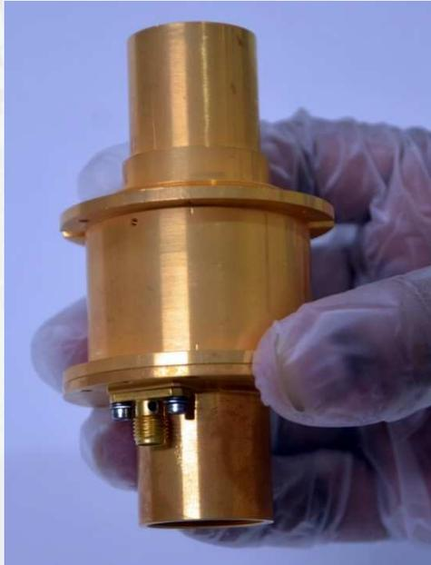
Jaydeep Kaintura et al, "Optics Integrated Compact Cavity for Rubidium Atomic Frequency Standards", Review of Scientific Instruments, vol. 90, 084701, 2019.
