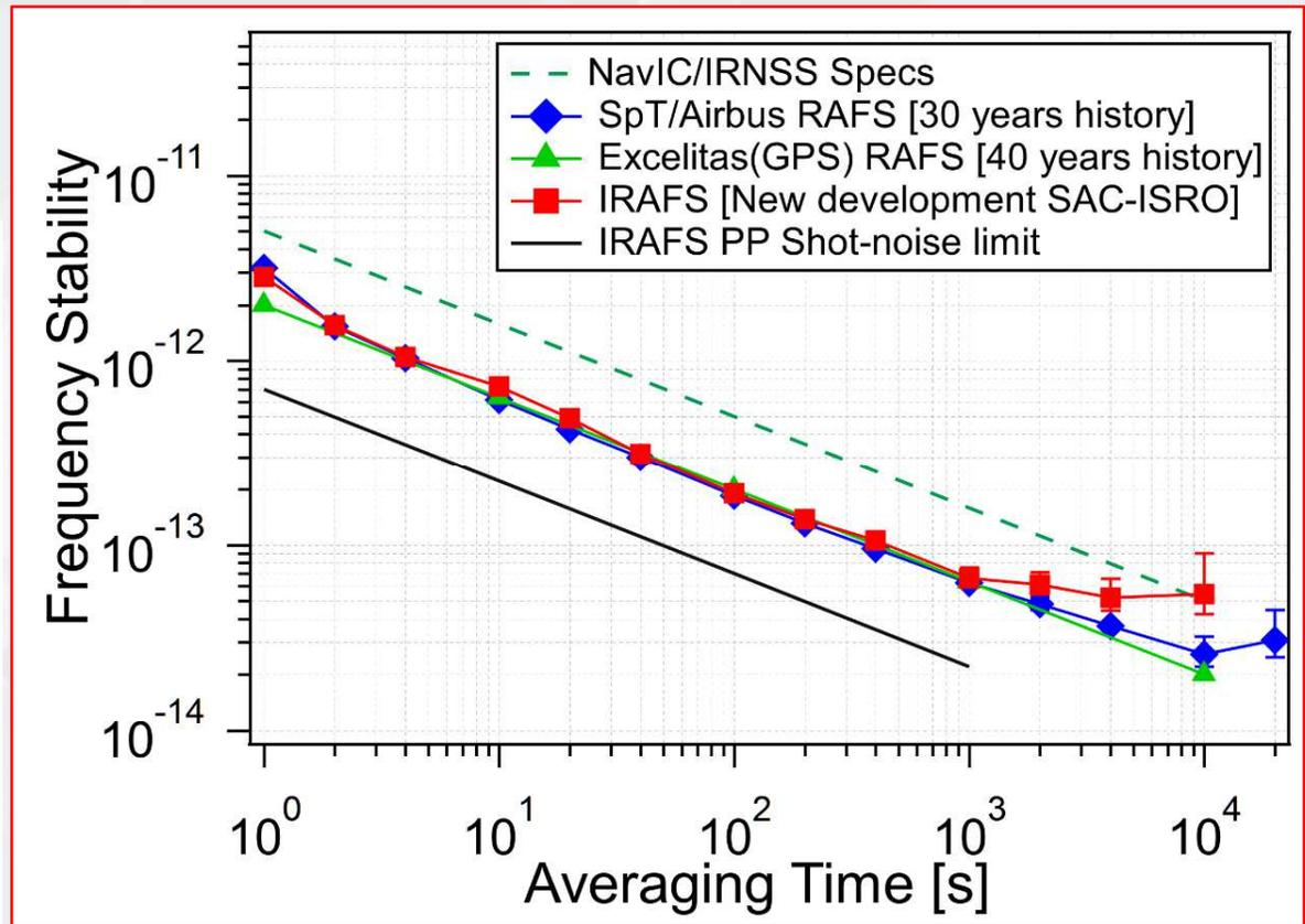
*Measured stability performance of IRAFS, also shown are IRNSS specifications and shot-noise limit of the Physics Package.*
