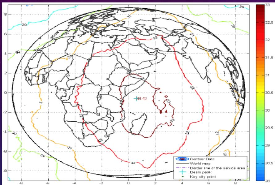
The downlink coverage beam of NIGCOMSAT-1R
