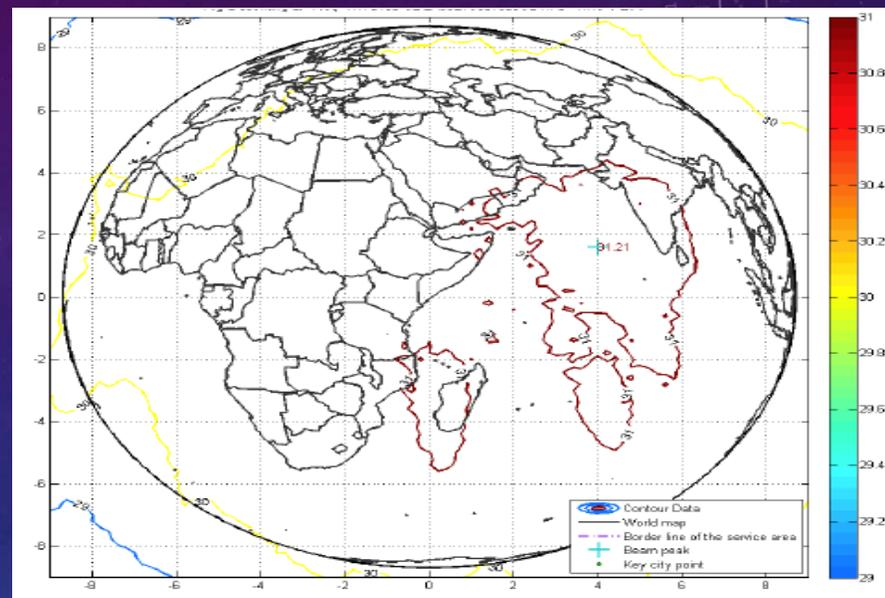
The downlink coverage beam of NIGCOMSAT-1R
