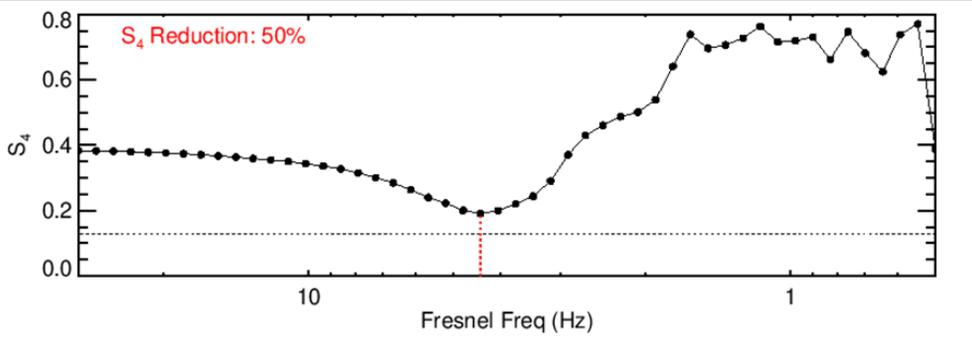
2. Geometric model provides Fresnel frequency vs distance. Intersection with measurement gives distance to irregularities.
