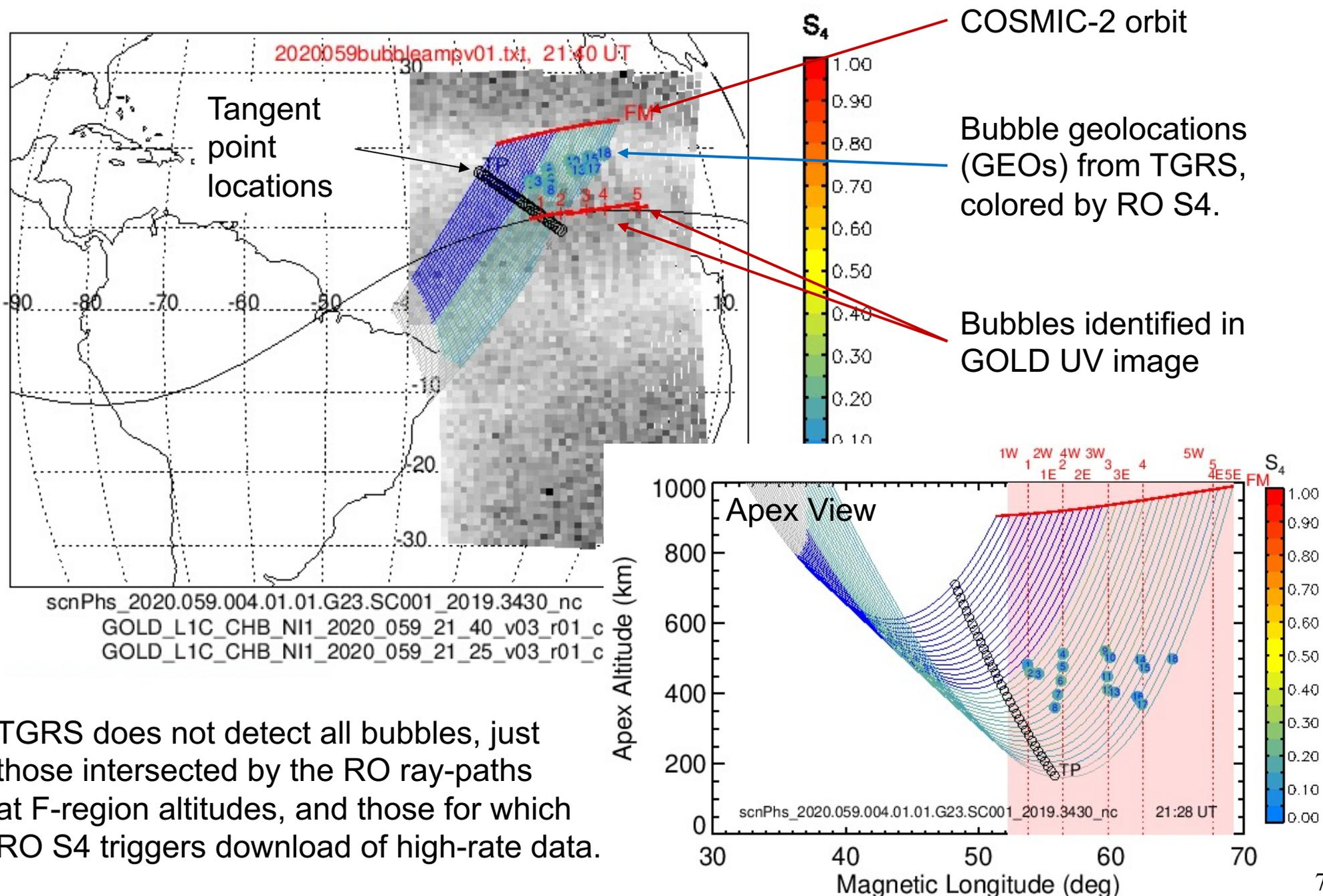
TGRS does not detect all bubbles, just those intersected by the RO ray-paths at F-region altitudes, and those for which RO  $S_4$  triggers download of high-rate data.
