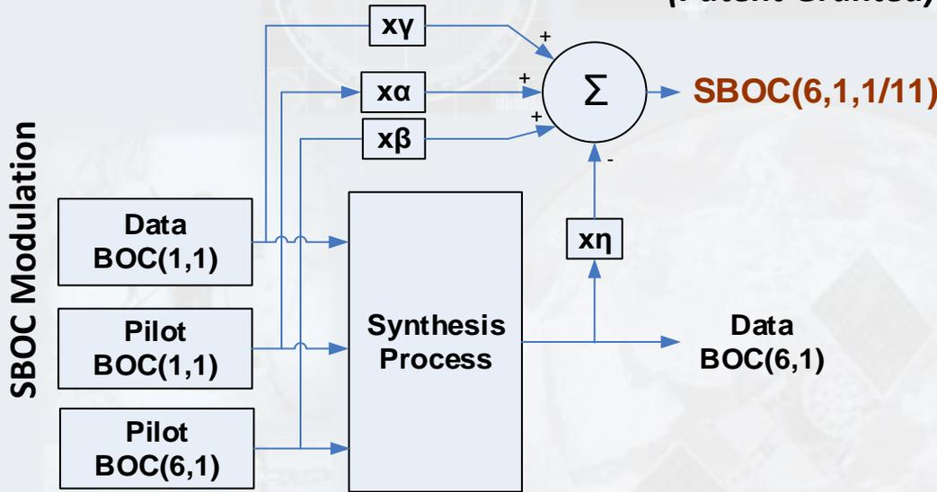
$$SBOC: S(t) = [\alpha S_{p1}(t) - \beta S_{p2}(t)] + j[\gamma S_{d1}(t) + \eta S_{p1}(t)S_{p2}(t)S_{d1}(t)]$$
