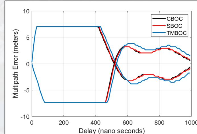
**Narrow band Rx. Multipath Perf. (0.05 chip spacing)**
