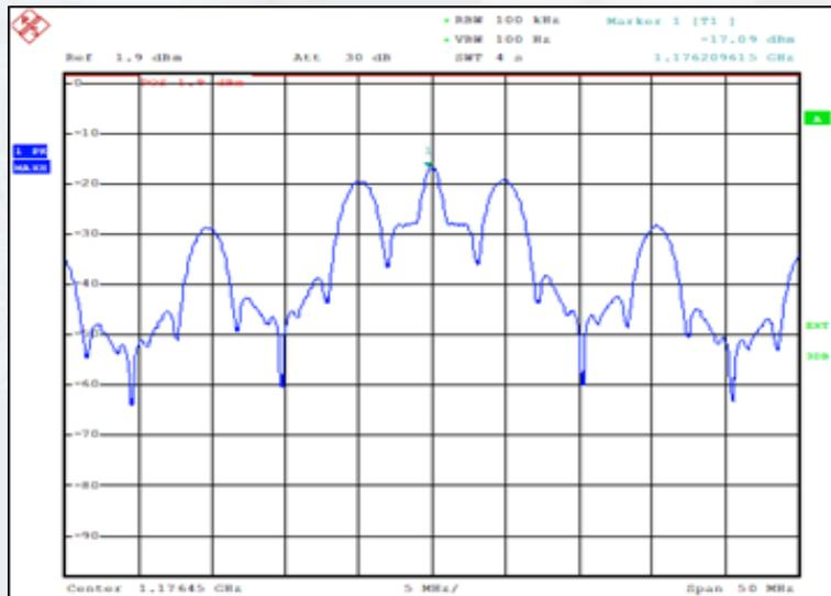
Measured Spectrum of Composite Signal
