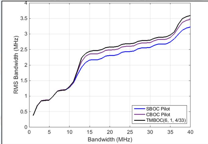
**RMS Bandwidth vs Receiver Bandwidth**
