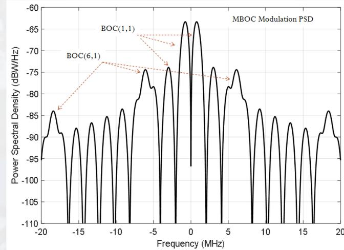
**NavIC New L1 band SPS (SBOC) Signal Spectrum**
