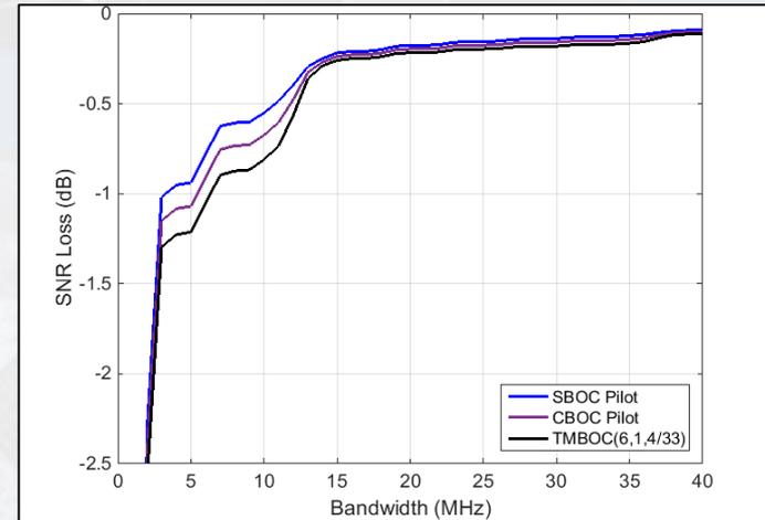
**SNR Loss vs Receiver Bandwidth**
