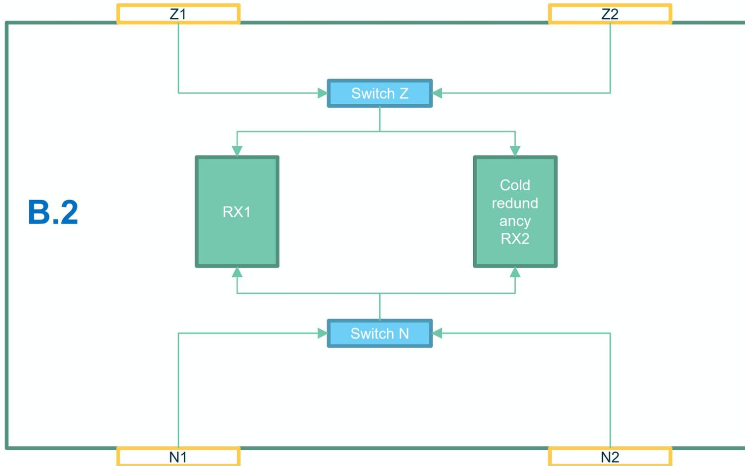
With redundant GNSS Zenit and NADIR antennas
