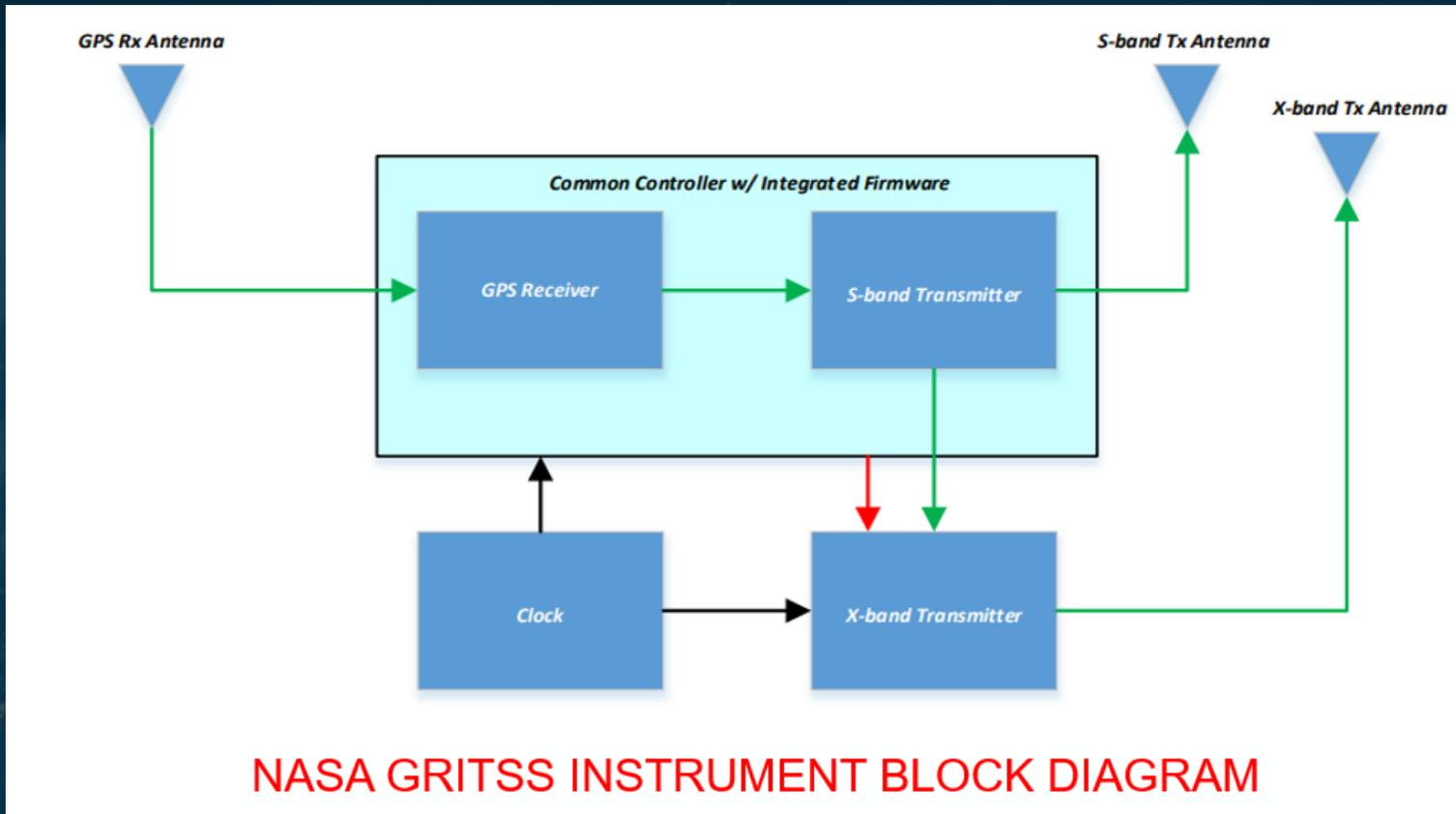
Transponding GPS to VLBI users over S and X-bands to enhance GNSS/VLBI collocation ties accuracy
