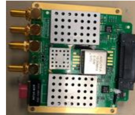
NC3m GNSS RF card(~3.5"x3.5")
