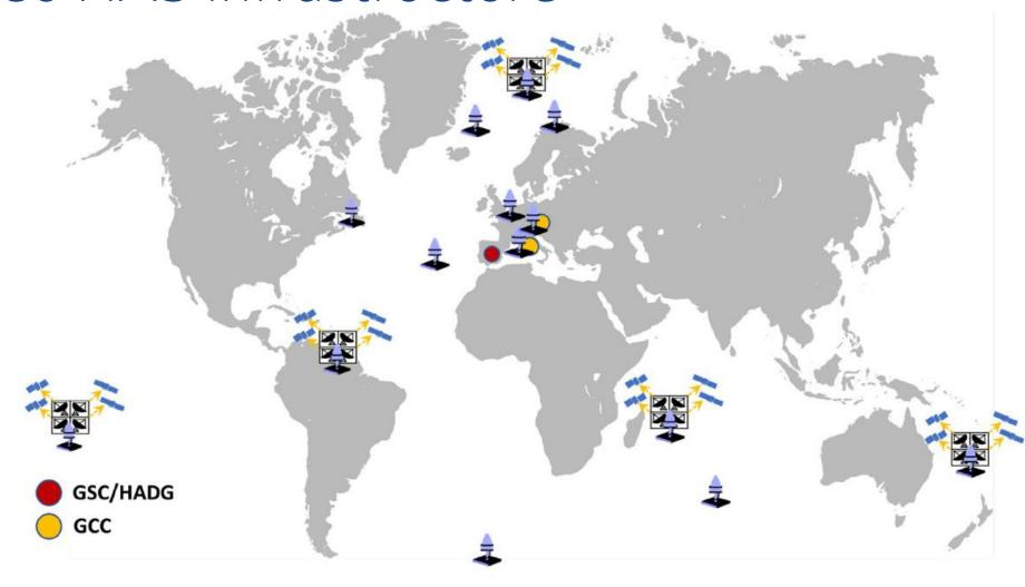
Galileo HAS Phase 1 architecture. The 14 GSS (Galileo Sensor Stations) are depicted with a single antenna, and the five ULS (Up-Link stations) are depicted with four antennas
