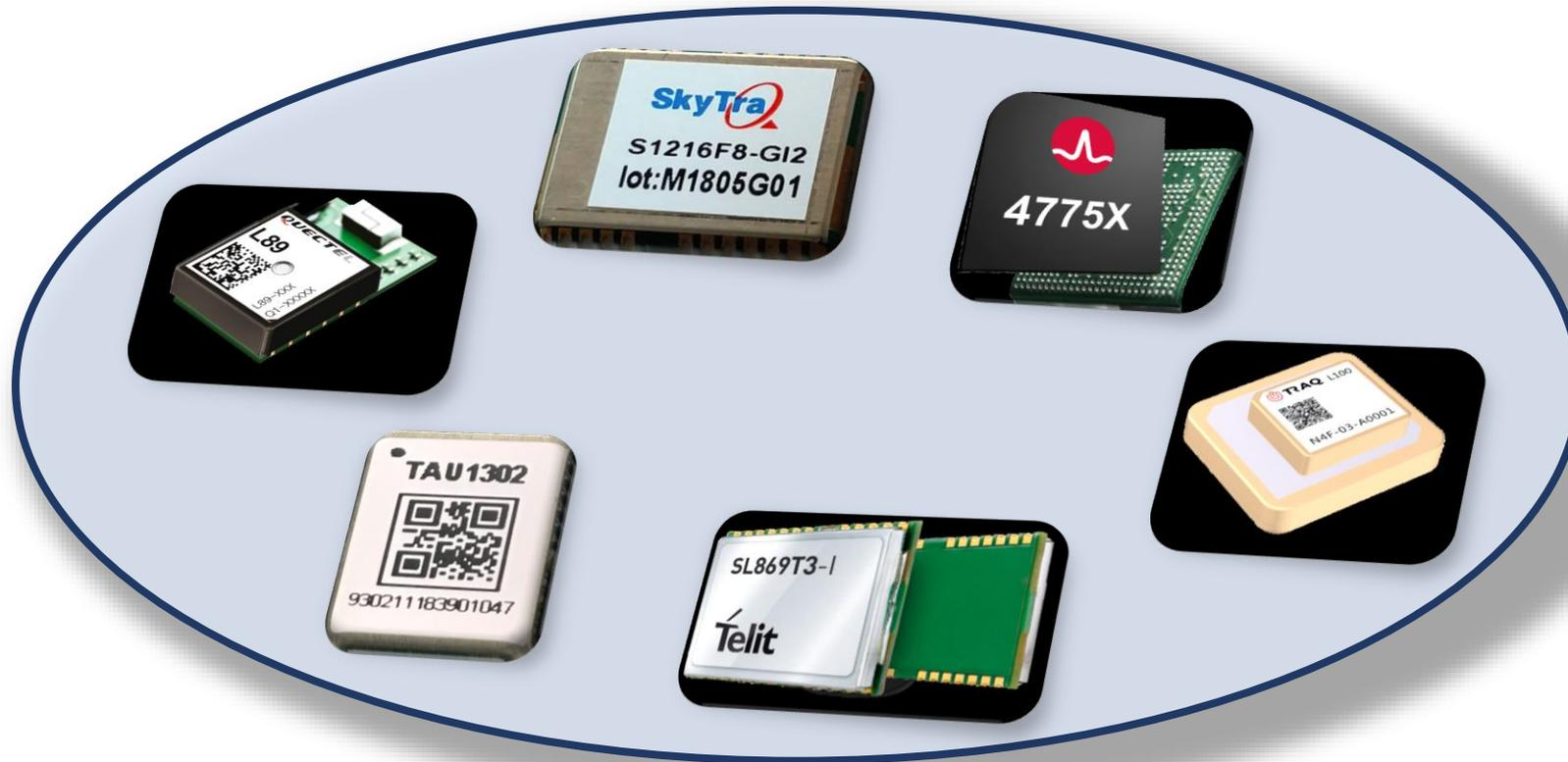
**A few of the off-the-shelf chips for standalone GNSS (NavIC enabled):
