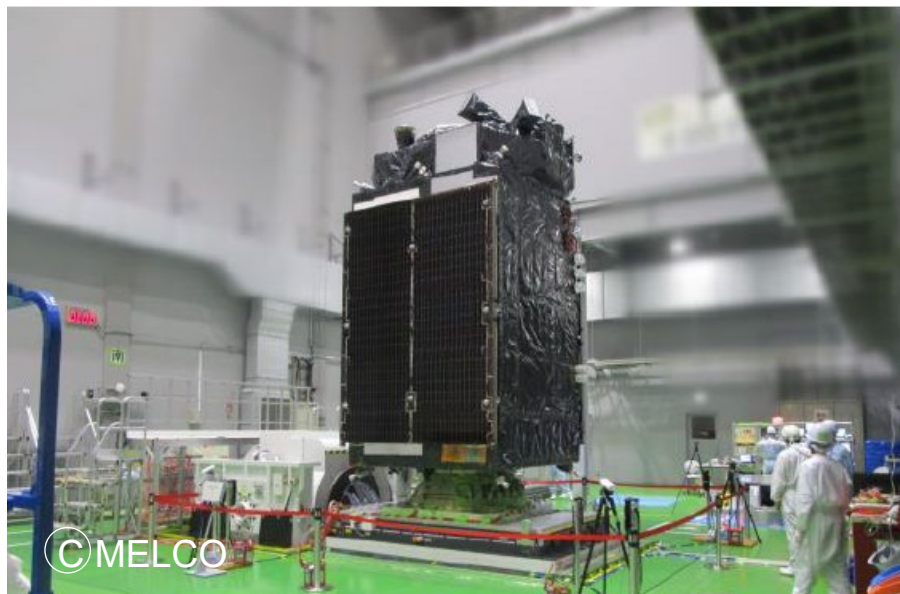
During the vibration test (X-axis) for QZS-5
