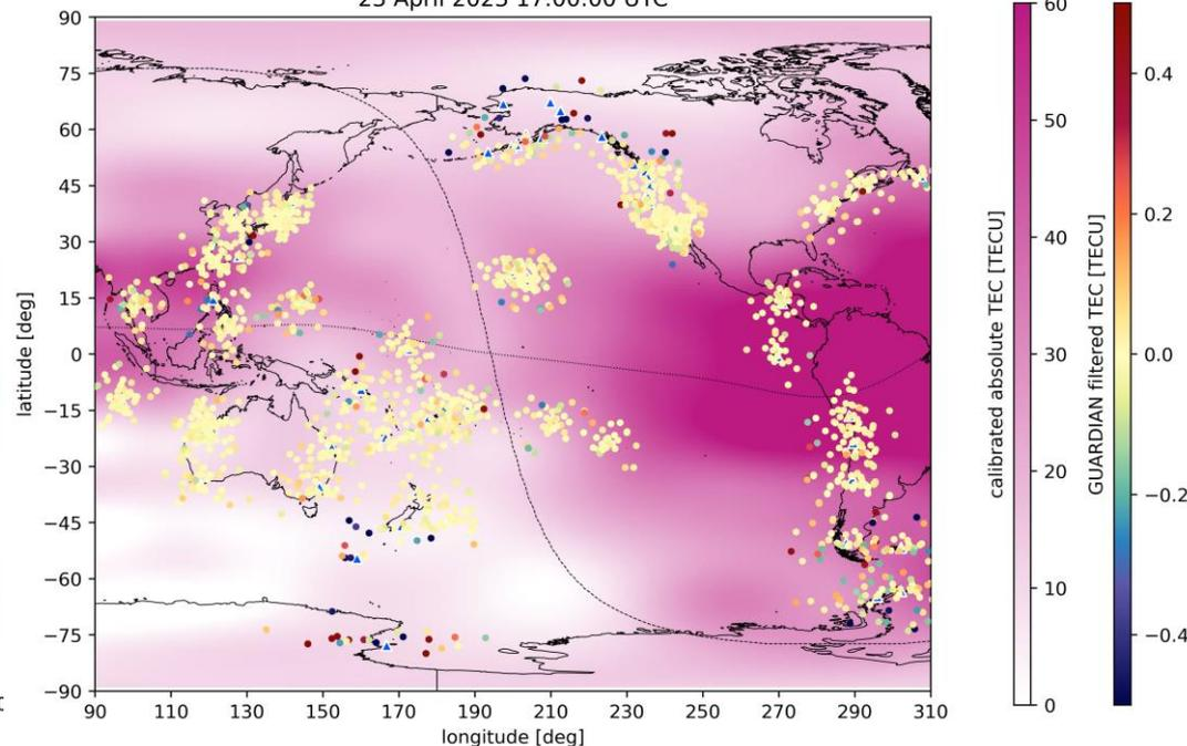
Real-time monitoring of ionospheric disturbances using a combination of high-resolution multi-shell GIM mapping and real-time GDGPS-based TEC measurements
