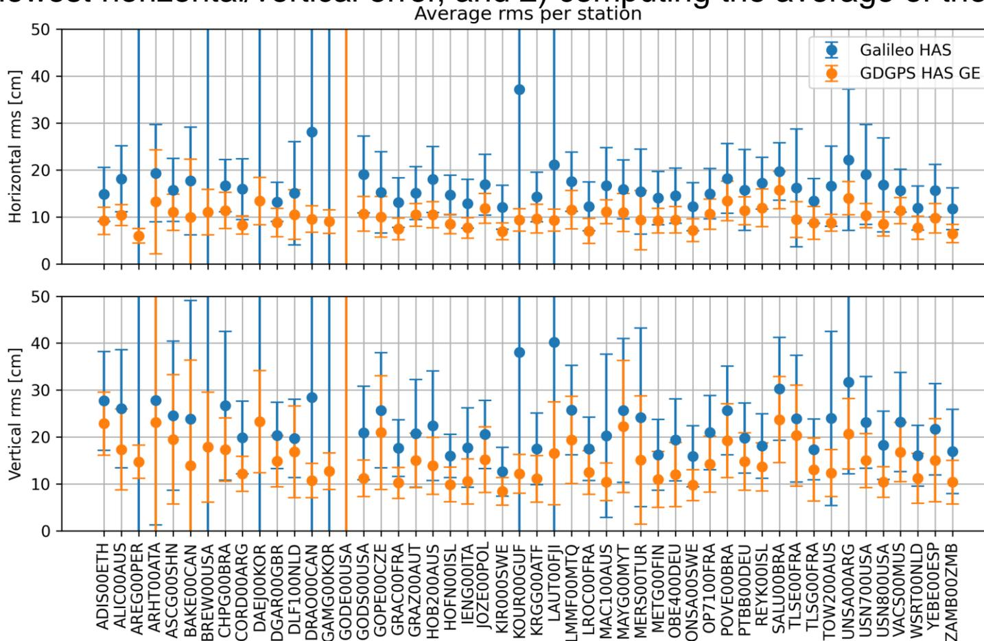
Average and 1-sigma error bars of RMS for horizontal and vertical components for individual stations investigated
