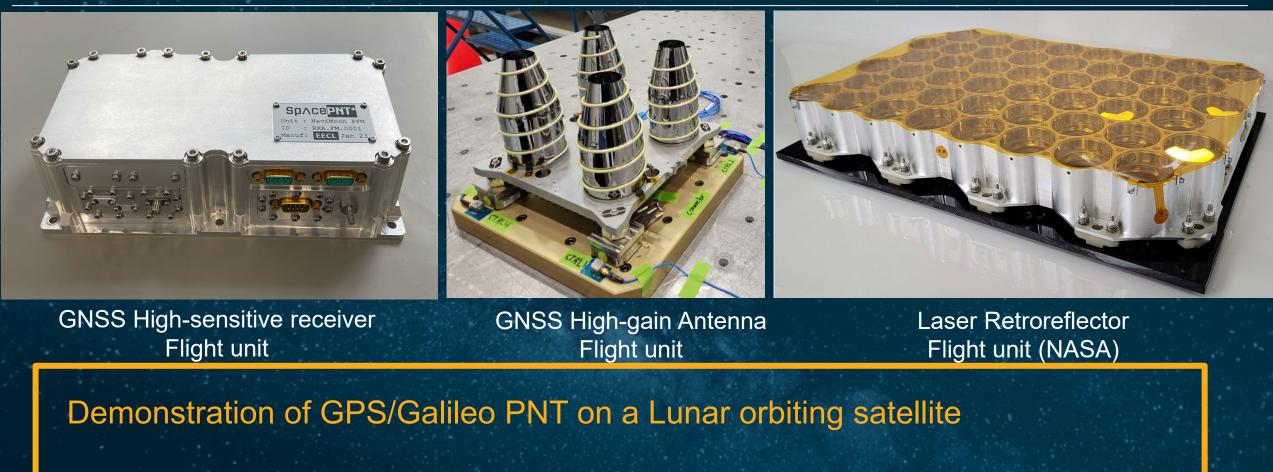
First time ever three ranging techniques (GNSS, Laser and X-band ranging) are used simultaneously on lunar orbit
