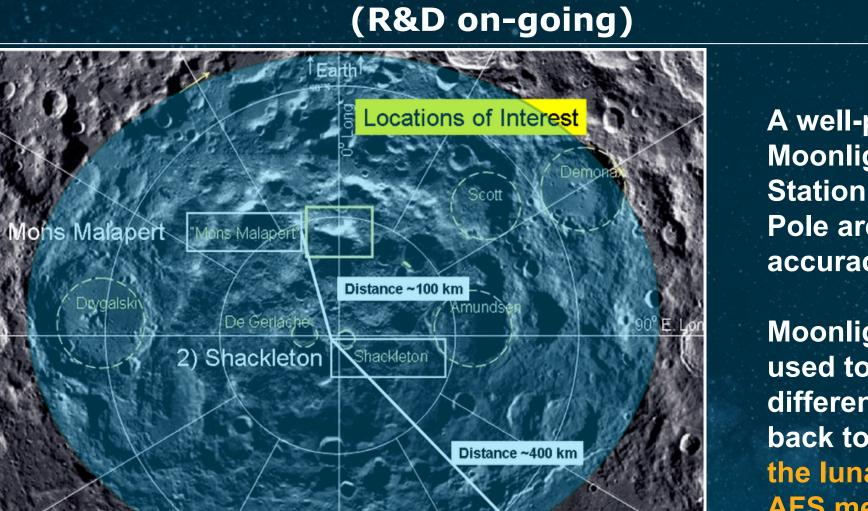
A well-placed single Moonlight LCNS Differential Station could serve all South Pole area allowing sub-metre accuracies in real time.
