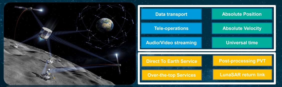
• A dedicated constellation of satellites around the Moon providing commercial lunar communication and navigation services in two steps IOC (2028) and FOC (2030).
