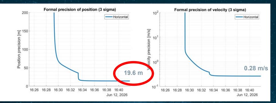
Combining Moonlight LCNS signals with a simple IMU and altimeter the achieved final landing horizontal precision obtained is <u>around 20 m !!</u> (bellow 50 m Spec)
