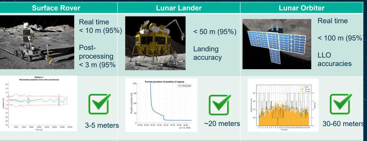
Ref: Navigation Performance of a Lunar Surface Rover Using LCNS Positioning Assuming Realistic ODTS Performances, EUROPEAN NAVIGATION CONFERENCE 2023 Ref: <u>Positioning and Velocity Performance Levels for a Lunar</u> Lander using a Dedicated Lunar Communication and Navigation <u>System</u>, Navigation Journal 2022 Ref: Navigation performance of Low Lunar Orbit satellites using a Lunar Radio Navigation Satellite System, ION-GNSS 2023
