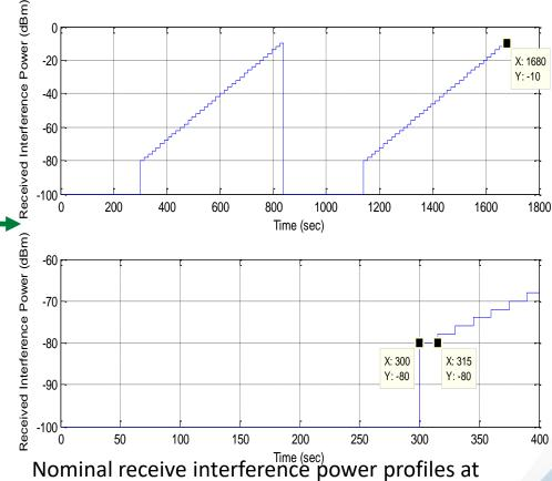
GNSS antenna location for the (1475 to 1540 MHz) and (1630 to 1675 MHz) frequency ranges.
