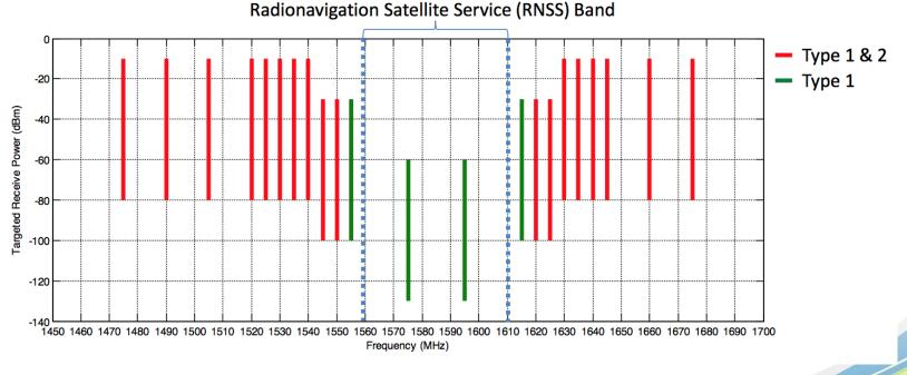
Interference Test Signal Frequencies and Power Profiles
