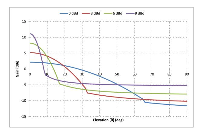
NOTE: Antenna gain is defined as the gain at  $0^0$  elevation angle.
