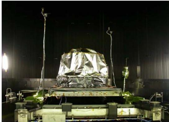
Thermal Vacuum Test of L-band Antenna Engineering Model (February 2007) 【MEXT】
