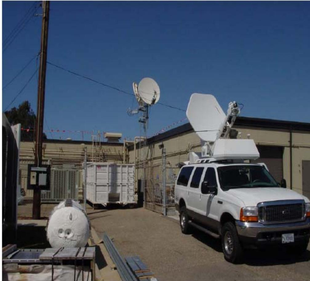
**Mobile / transportable TWSTFT station provides time transfer accuracy: 1ns**
