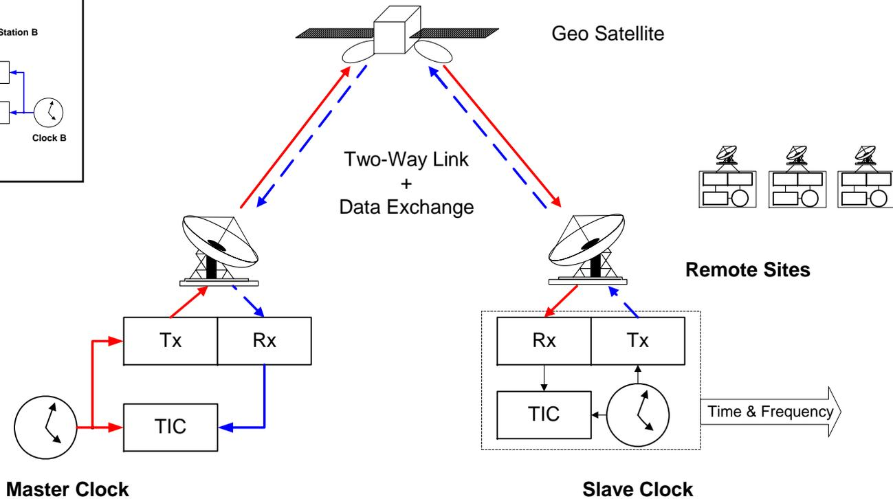
**TWSTFT-based time synchronisation of a slave clock to master site
