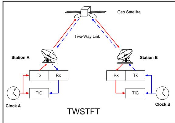
**TWSTFT used to link primary clocks, time-to-alarm: < 3s
