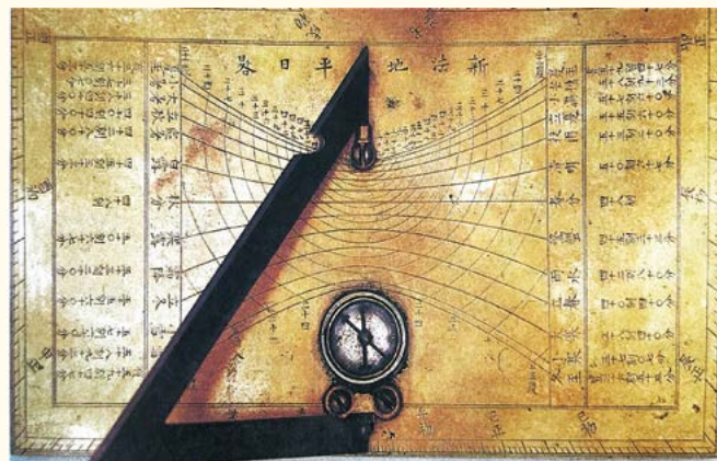
新法地平日晷（上）及晷面图（下），现存于故宫博物院 Horizontal Sundial with the New Mechanism (top) and the dial plate (bottom), currently in the Palace Museum
