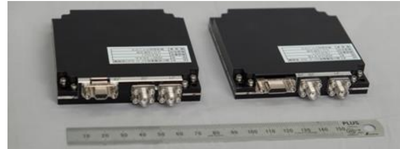
Typical CubeSat RF Transmitter and Receiver © Addnics corp.
