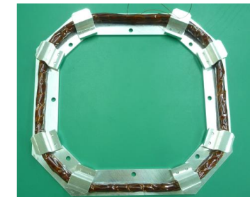
Magnetic Torquers (Electrical Coil)
