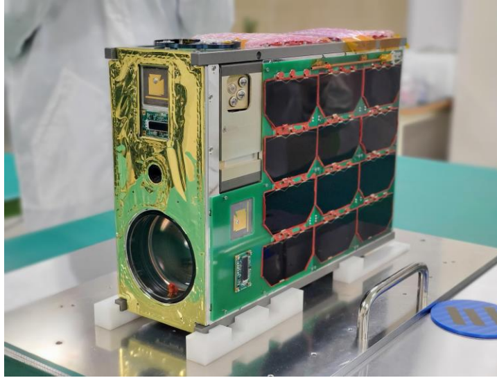
6U based on BIRDS-3/4 High power + Li-ion battery High speed communication Active attitude control
