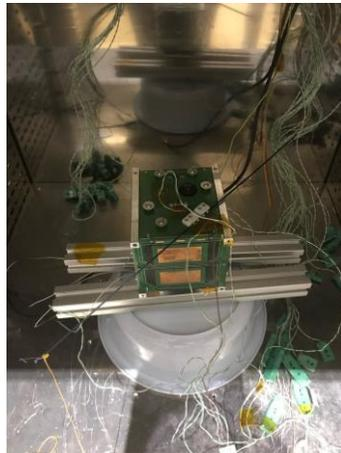
Antenna deployment in very cold temperature
