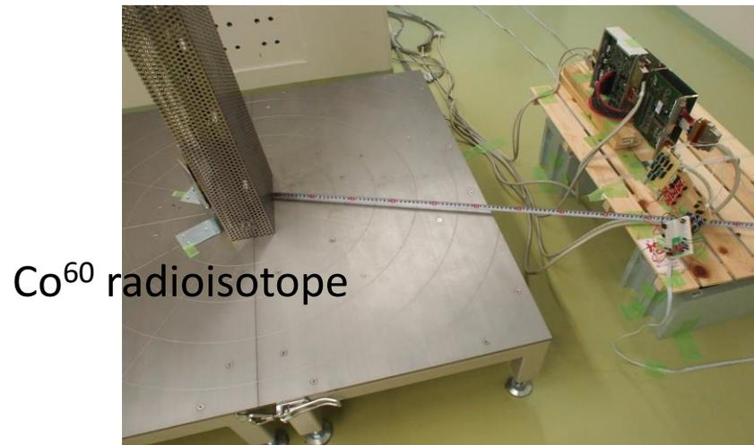
Confirm that the hardware (electronic parts) can survive ionizing radiation
