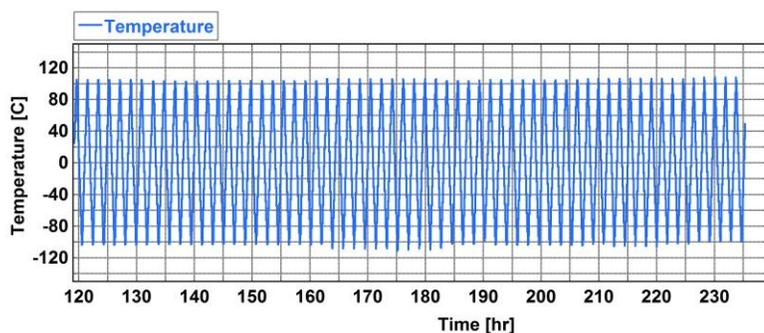
Confirm that the hardware can survive repeated cycles of hot and cold temperature
