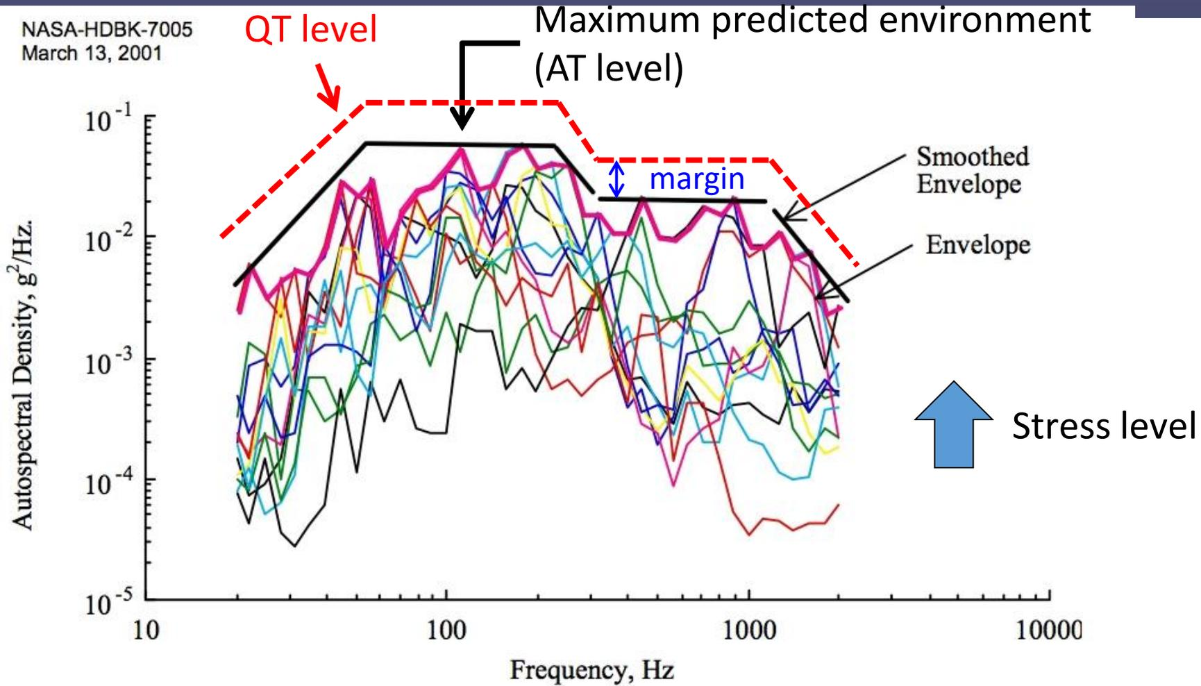
FIGURE 6.1. Envelope for Twelve Measured Vibration Response Spectra Within a Zone.
