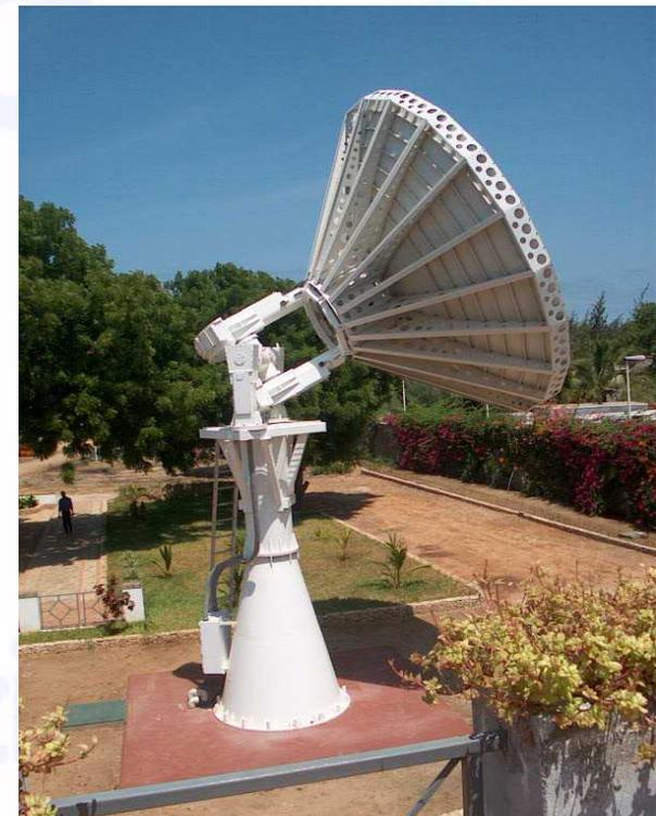
The Remote Sensing Centre at the BSC acquires EO satellite images both in L-band and in X-band. An average of 12 to 15 images per day are acquired from different sensors, processed and archived. The 6.2 m antenna in X-band is used to acquire MODIS/Terra and MODIS/Aqua
