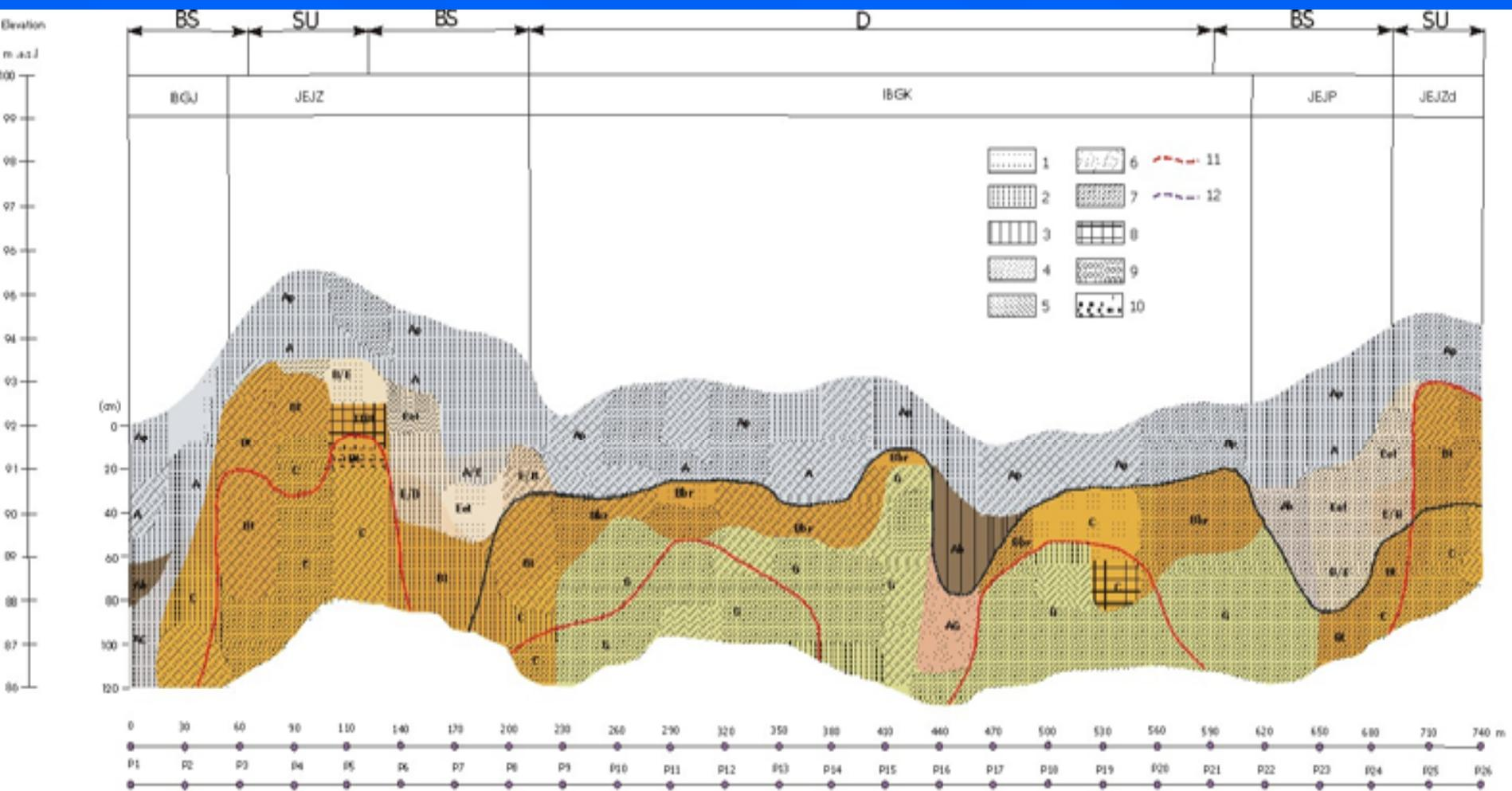
Pedagogical cross-section AB - Pólka: 1 - sand, 2 - loamy sand, 3 - loamy fine sand, 4 - sandy loam, 5 - sandy clay loam, 6 - loam, 7 - fine sandy loam, 8 - coarse sand, 9 - very fine sand, 10 - coarse sandy loam, 11 - top of calcium carbonate accumulation, 12 - top of gley spots, P - profile, D - depression, BS - backslope, SU - summit, IBGK - Typic Endoaquolls, IBGJ - Fluvaquentic Endoaquolls, JEJZ - Glossic Hapludalfs, JEJP - Glossic Hapludalfs, JEJZd - Typic Hapludalfs
