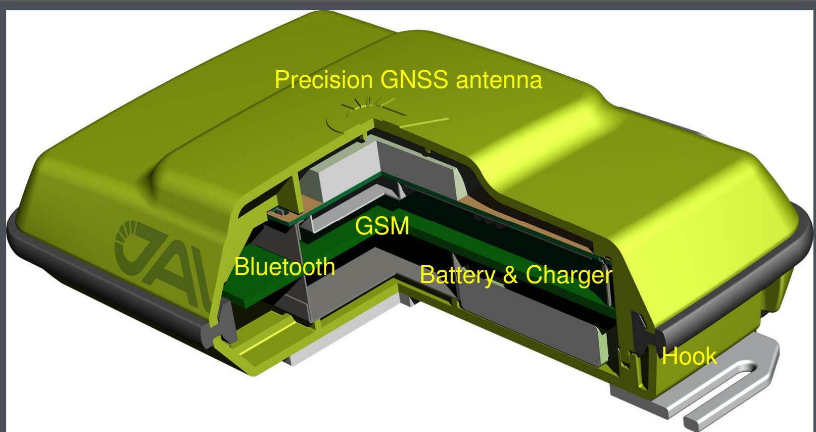
32 channels of GPS and GLONASS L1, code and carrier
