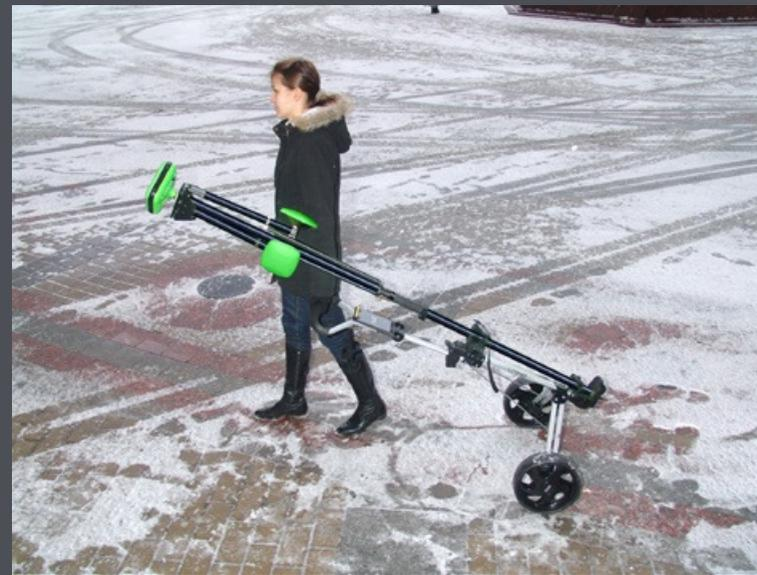
To make handling of the three additional antennas easy we have designed the RTK Umbrella. The receiver is mounted in the center and three small antennas on three folding arms. We took the hint from golfers and offer a modified golf caddy. The RTK Caddy is easy to store, transport and use in the field. It is especially helpful when roving with TRIUMPH-4X.
