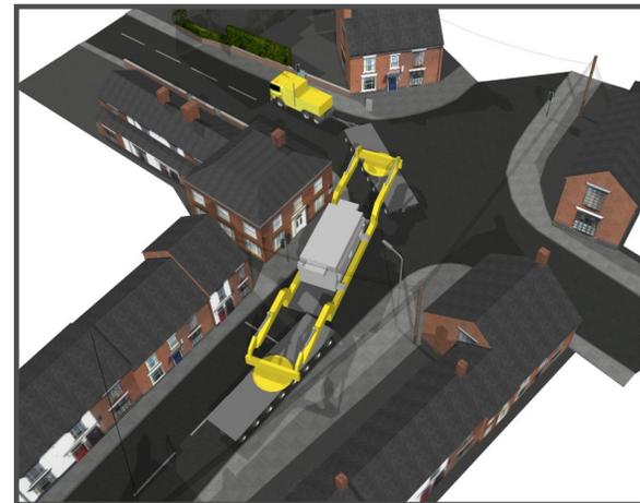
*Application 4 – Point cloud and CAD model for an intersection; 3D model used in the route study © 3DLM*
