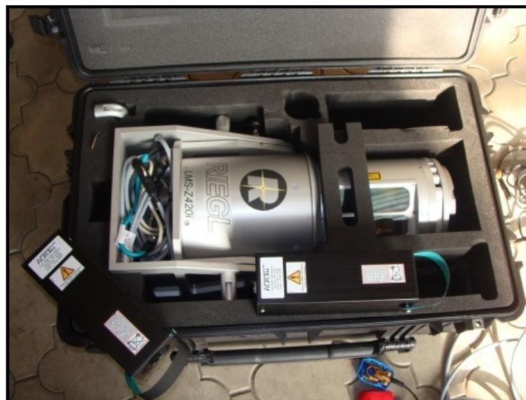
Riegl LMS Z420i laser scanner used by
