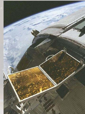
PLATAN (PLASTIC TRACK ANALYZER) – multilayer lavsan based detector
