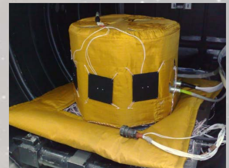
Outer detectors of Photon-Gamma apparatus in the thermo vacuum test chamber
