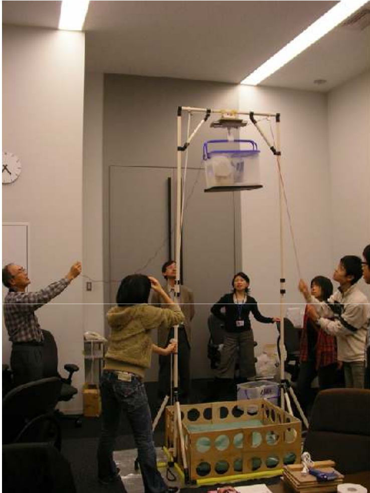
2-meter/0.6-second drop test tower constructed by JAXA
