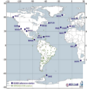
Fig. 1. IGS05 reference stations applied for the datum realization.
