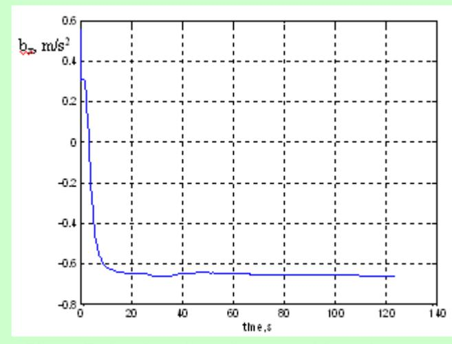
Fig. 4. Estimation of accelerometer bias, when  $v=60$  km/h
