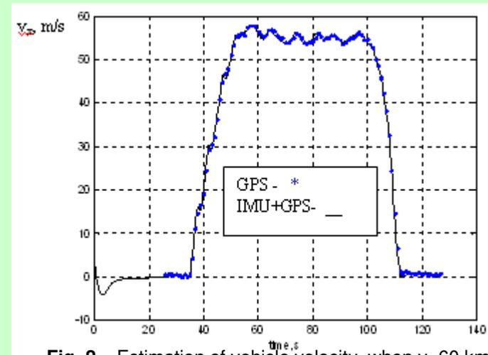
Fig. 2. Estimation of vehicle velocity, when  $v=60$  km/h
