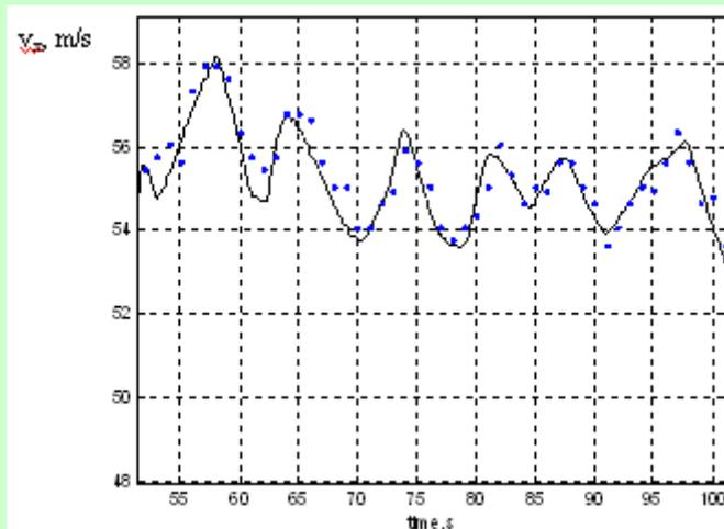
Fig. 3. Estimation of vehicle velocity, when  $v=60$  km/h (zooming in of the Fig.2 at time interval from  $t= 50$ s till  $t=100$  s)
