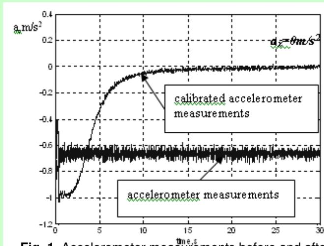
Fig. 1. Accelerometer measurements before and after postcalibration process
