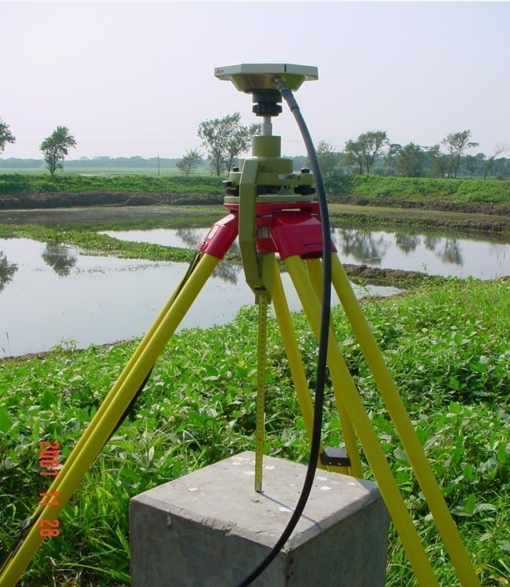
□ Dual frequency Geodetic Grade GNSS Receiver were used for both 1<sup>st</sup> Order and 2<sup>nd</sup> Order observations
