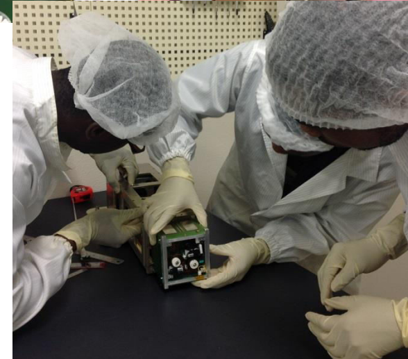
Structure Assembly and Fit check Acceptance Test
