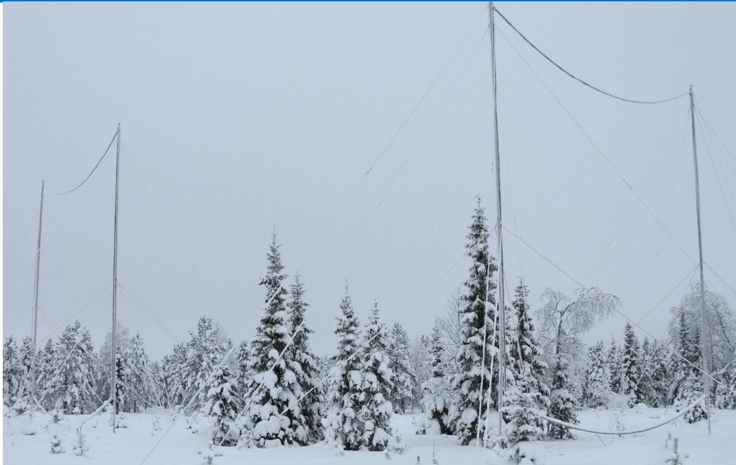
Two square loop antennas of 10m by side
