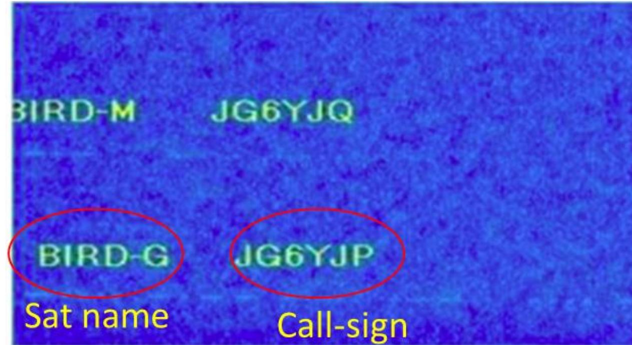
GhanaSat-1 signal reception decoded by Software Define Radio Interface
