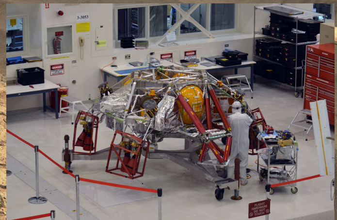
Mar 13, 2018 - A technician works on the descent stage for NASA's Mars 2020 mission inside JPL's Spacecraft Assembly Facility
