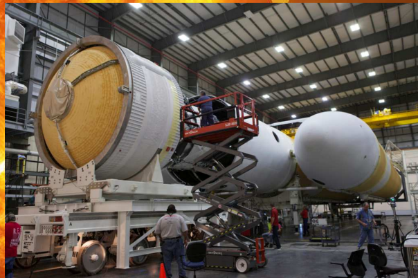
March 29, 2018 - Second stage of a United Launch Alliance Delta IV Heavy is mated to the common booster core at Cape Canaveral Air Force Station
