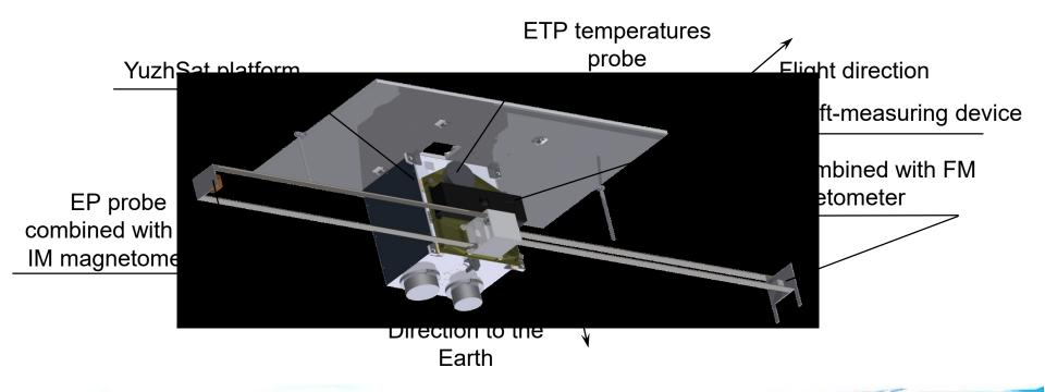
The Clusterion is a perspective project that will provide new quality of study of the dynamic links in the "atmosphere-ionosphere-magnetosphere" system by carrying out the multi-point synchronous measurements of the ionosphere plasma parameters using a cluster of 2 ... 4 microsatellites based on the YuzhSat - magnetically clean platform. It is planned to install the Clusterion scientific equipment on the spacecraft.
