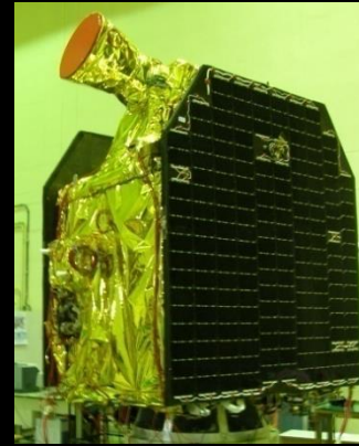
SOLAR PANELS STOWED
