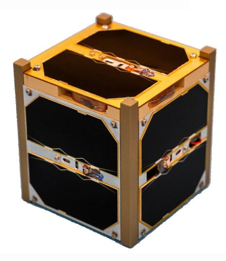
A "standard 1U" CubeSat has a volume of one liter -10 cm cube and a mass of 1 kg, orbiting at 300-600 km circular orbit, 1W transmitter on 145 MHz or 435 MHz amateur-satellite service bands. It's used for academic education, research and technology validation applications but also for complex science and governmental use.
